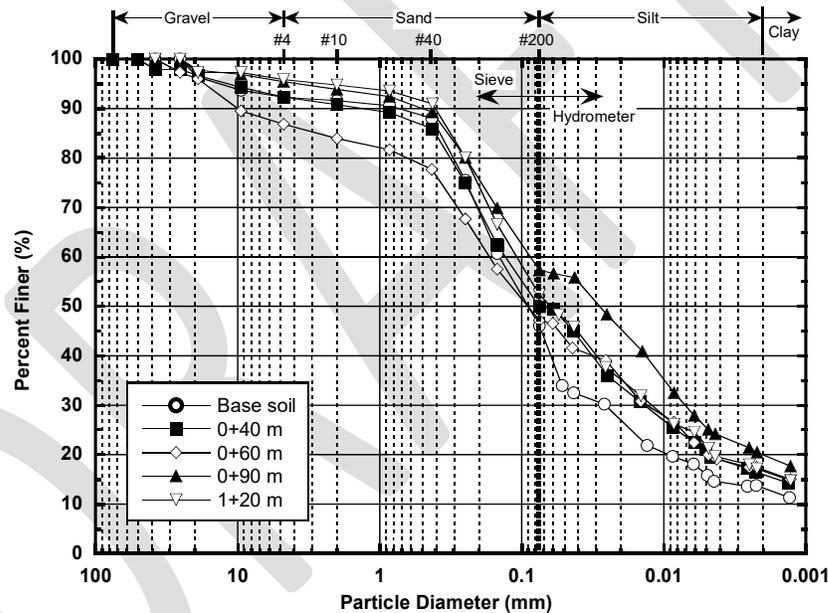
**Fig. 2. Grain size distribution of base soil and backfill (legend indicates station of backfill sample).**
