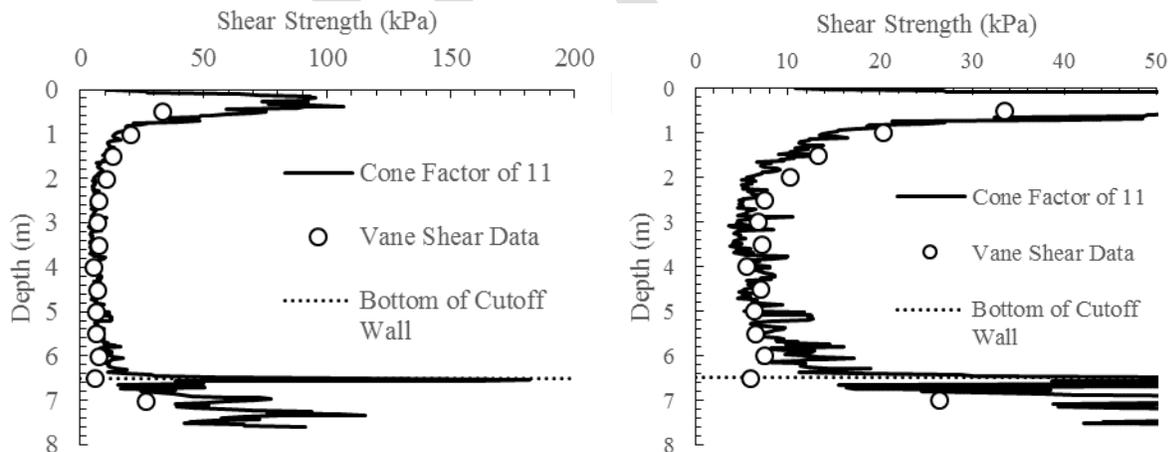
**Fig. 4. Shear Strength vs Depth of Cutoff Wall**
