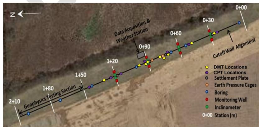
**Fig. 1. Plan view of the cutoff wall with instrumentation and CPT/DMT testing locations.**
