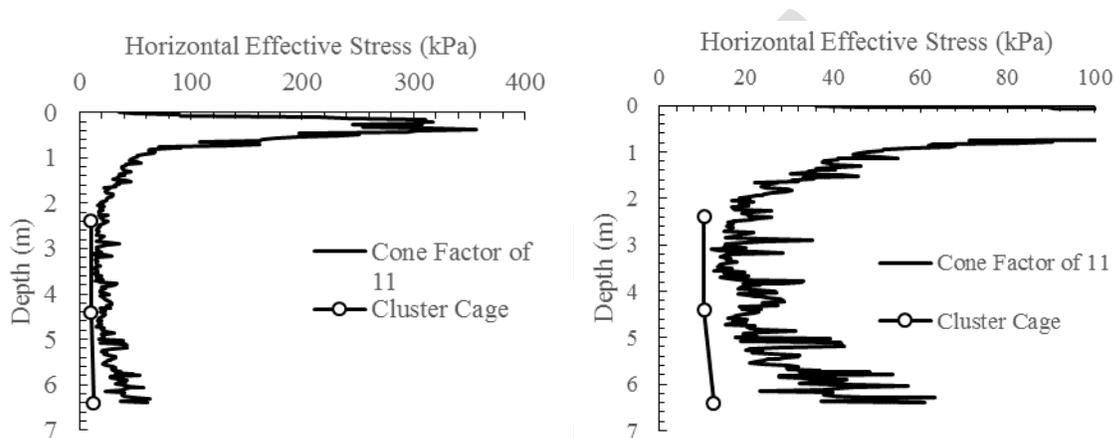
**Fig. 5. Horizontal Effective Stress ( $S_u/\sigma_h' = 0.3$ )**
