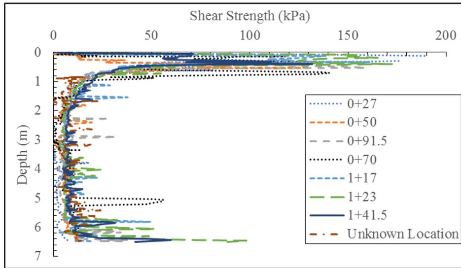
**Fig. 3. Shear Strength vs Depth of Cutoff Wall**
