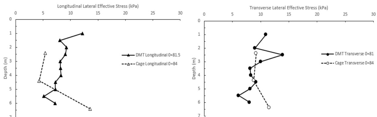
**Figure 8. Lateral Effective Stress at Specific Locations near Instrumentation Cages**
