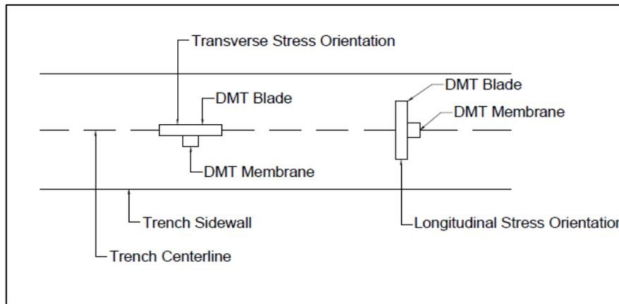
**Fig. 6. Transverse and Longitudinal Dilatometer Orientations (after Ruffing et al. 2011)**
