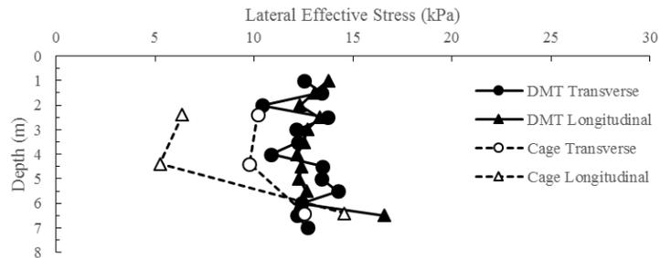
**Fig. 7. Lateral Effective Stress Averages from DMT and Instrumentation Cages**
