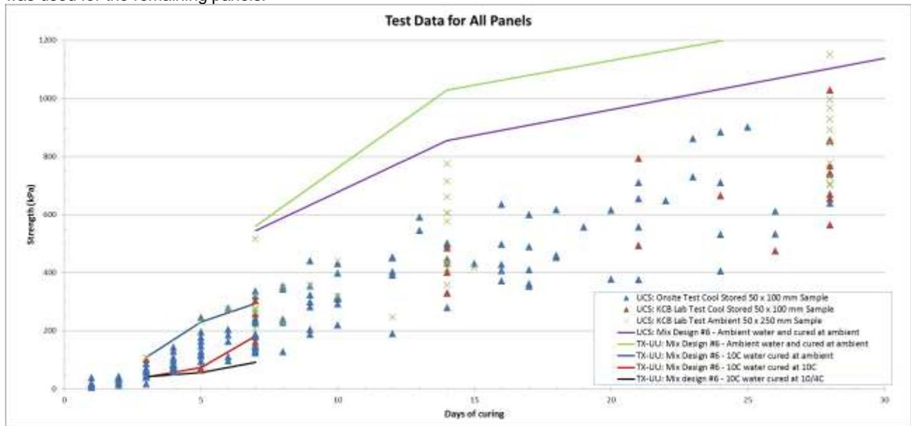
Figure 7. Graph showing comparison of strength results between cool stored and ambient stored samples, including design mix results.
