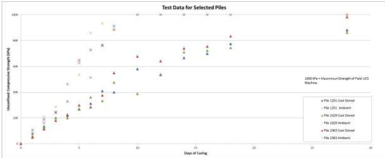
Figure 2. Increase in Strength for grout cured at different temperatures for the Continuous Flight Auger Cut-off Wall.
