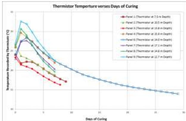
Figure 4. Graph of temperature trends measured by the thermistor which gave the overall lowest temperature in each panel.
