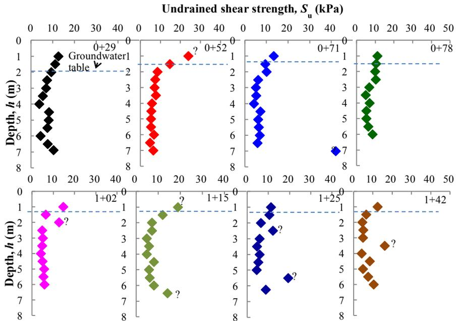
Fig. 3. Undrained shear strength at different test locations of the wall.
