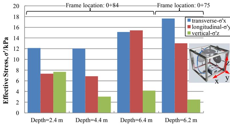
Fig. 5. Transverse, longitudinal, and vertical effective stresses at different depth in wall.
