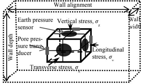
Fig. 2. Diagram of earth pressure cage installed within the trench wall.
