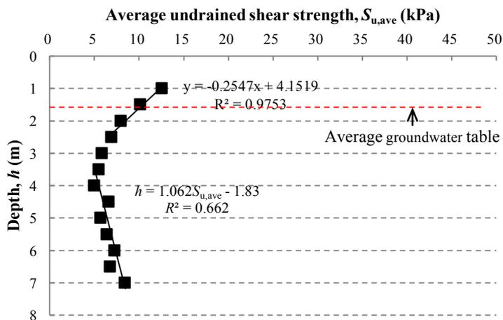
Fig. 4. Variation of average undrained shear strength with depth.
