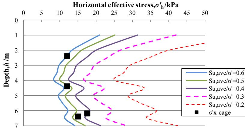
Fig. 6. Measured and predicted horizontal effective stress vs. depth.
