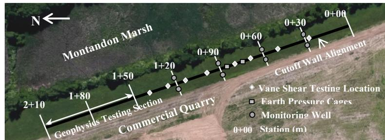
**Fig. 1.** Plan diagram of the cutoff wall with locations of the monitoring wells and the vane shear testing points.
