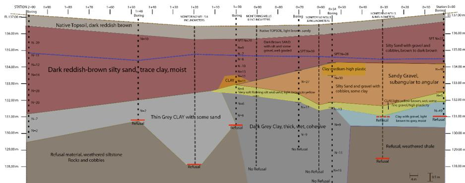
**Fig. 1.** Subsurface profile along the cutoff wall alignment based upon preconstruction investigations
