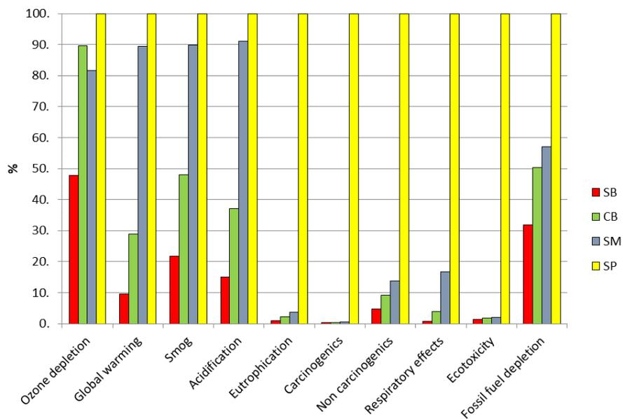
Fig. 3. Environmental impacts of the four vertical barrier systems across the midpoint impact categories of TRACI 2.1 LCIA method.
