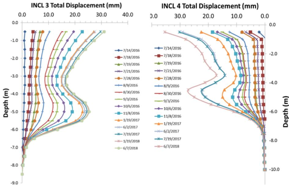
**Figure 3. Inclinometer deflections from inclinometer pair closest to the earth pressure measurements.**
