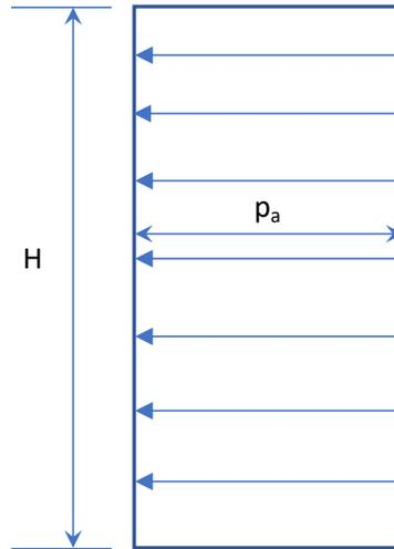
Fig. 4 Apparent earth pressure diagram for a braced cut in sand (After Peck 1969)
