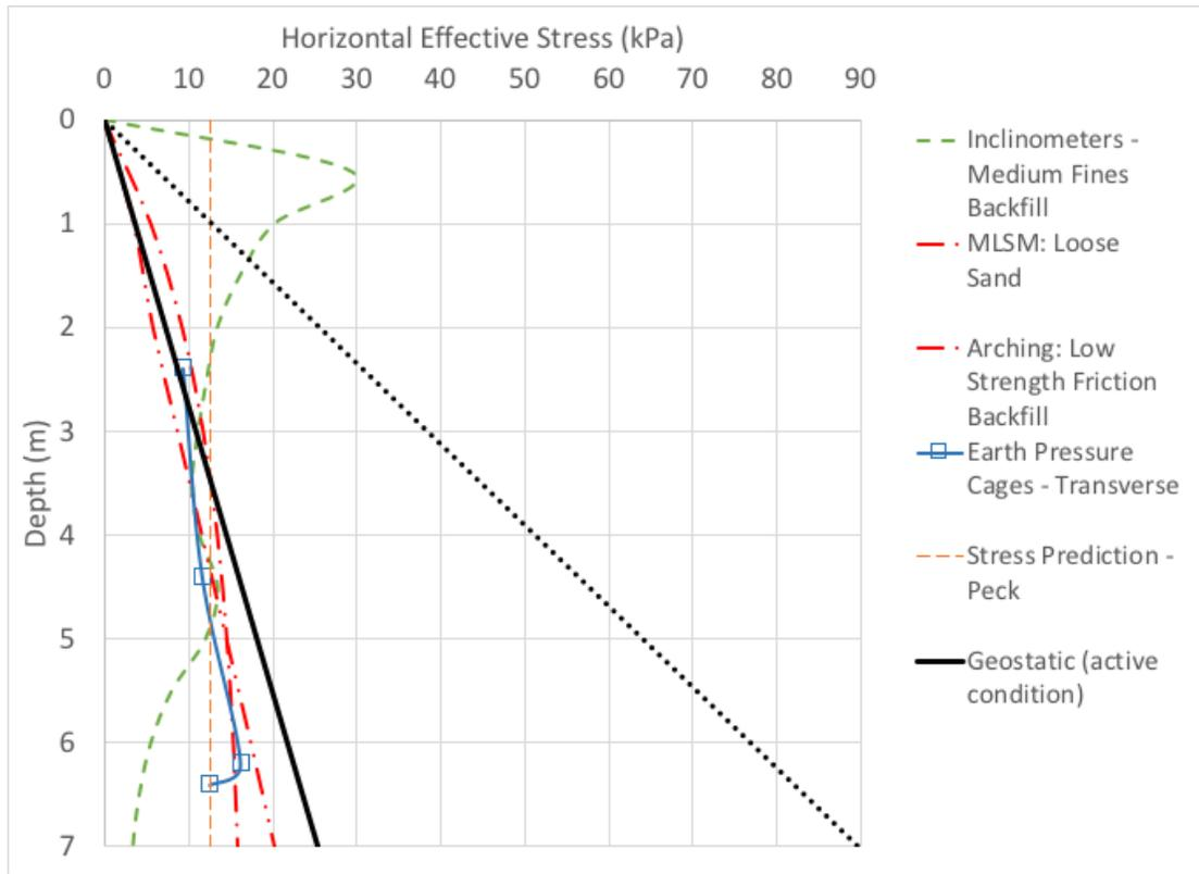
Figure 5. Stress Predictions and Measurements for the Subject SB Cutoff Wall.
