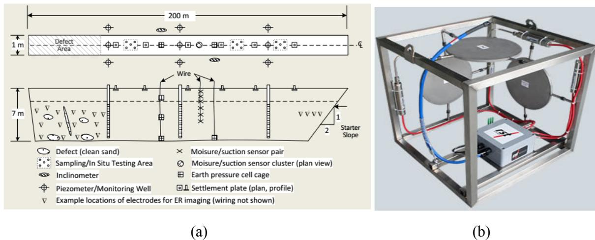
**Figure 1. (a) Plan and cross-section of SB wall with instrumentation. (b) Instrumentation cluster.**
