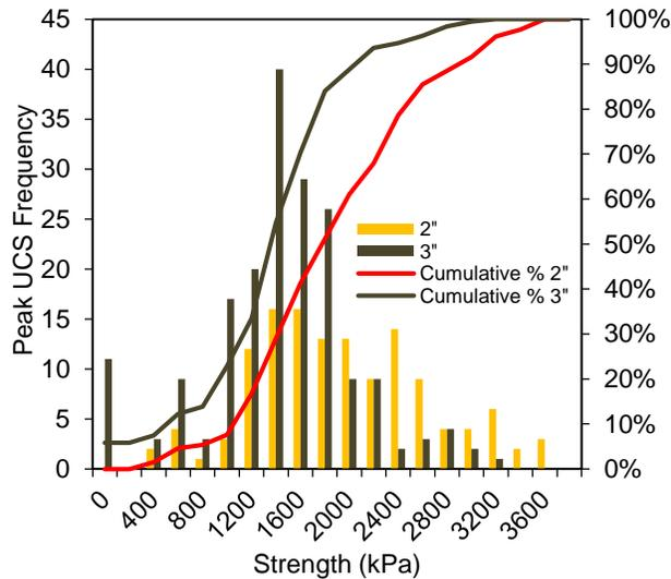
Figure 6. UCS Histogram of 3" vs 2" diameter samples
