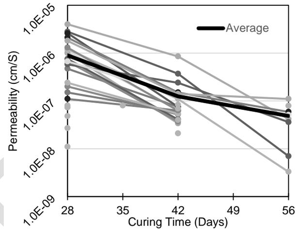
Figure 2. Hydraulic conductivity vs set-time of Slag-CB samples
