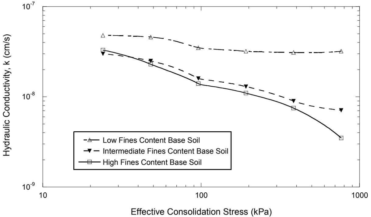
**Fig. 1. Effective stress vs.  $k$  for SB backfill (plotted from data in Evans and Huang 2016)**
