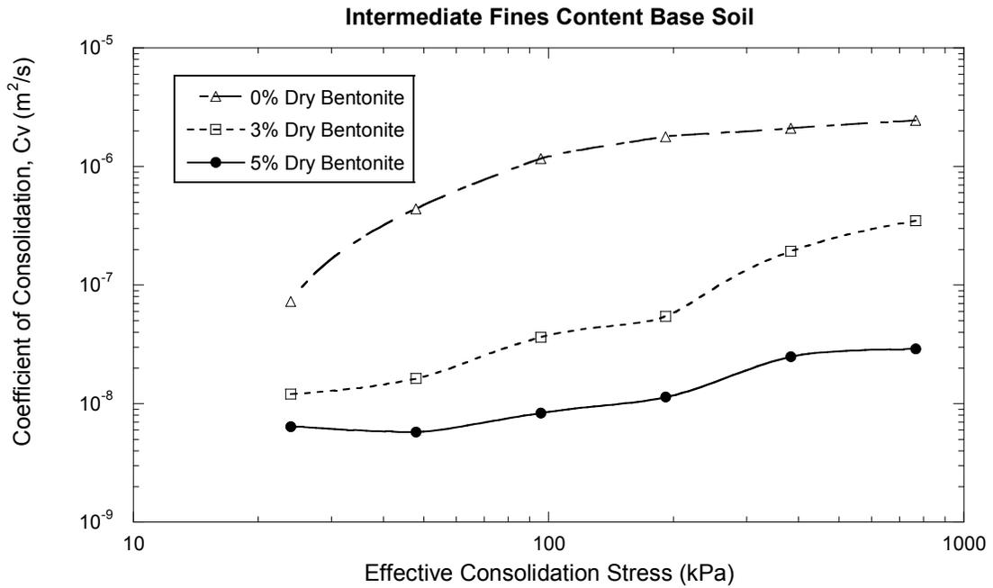
**Fig. 5. Coefficient of consolidation for intermediate fines content backfills**
