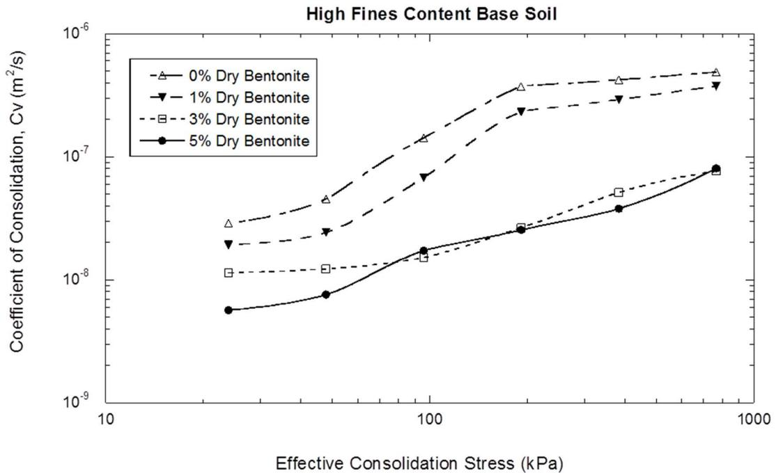
**Fig. 6. Coefficient of consolidation for high fines content backfills**
