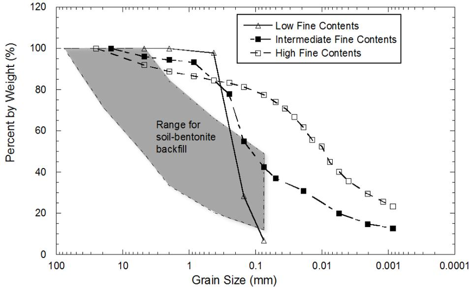
**Fig. 2. Grain Size of SB Soils and Recommended Range (from Evans and Huang 2016)**
