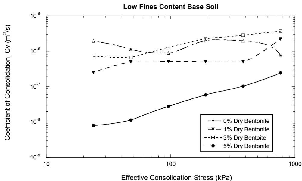
Fig. 4. Coefficient of consolidation for low fines content backfills
