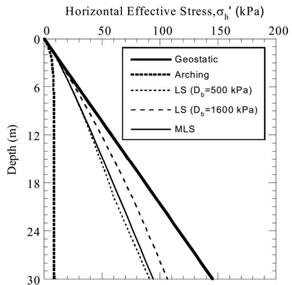
**Fig. 9. Horizontal effective stress distributions in SB cutoff wall ( $B = 1$  m) predicted by arching, lateral squeezing, and geostatic methods (from Fig. 6. in Ruffing et al. 2010)**
