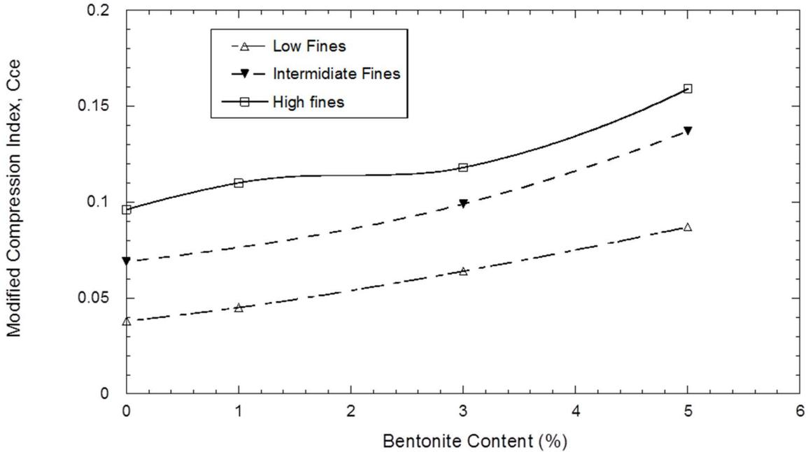
**Fig. 7. Modified compression index for backfills**
