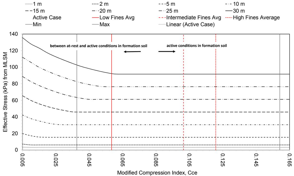
**FIG. 10. Horizontal stress as a function of modified compression index and depth for a theoretical medium dense sand ( $\phi=35^\circ$ ) formation soil**
