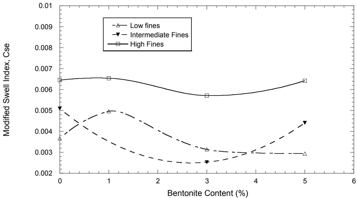
**Fig. 8. Modified swell (recompression) index for backfills**
