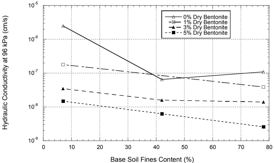
**Fig. 3. Base soil fines and dry bentonite vs.  $k$  of SB (from Evans and Huang 2016)**
