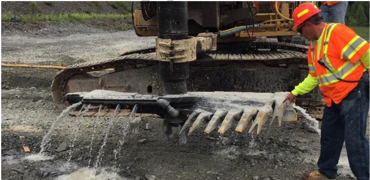
Figure 4. Large Diameter Auger with Grout Ports
