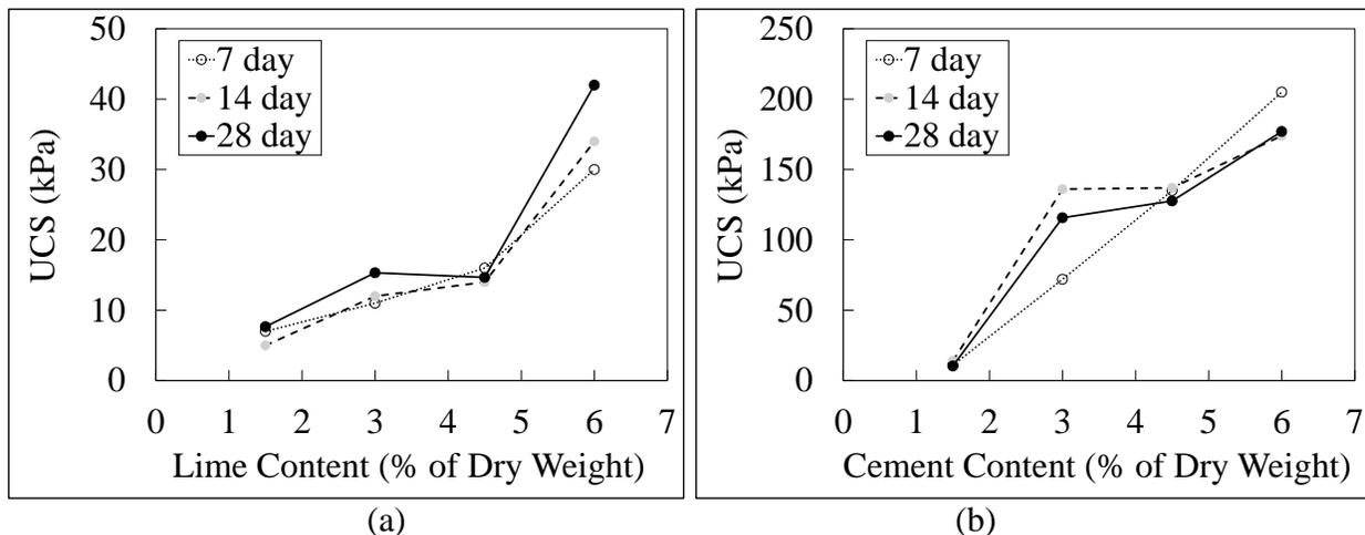
**Figure 1a. UCS of solidified fly ash vs. lime content and 1b. UCS of solidified fly ash vs. cement content**
