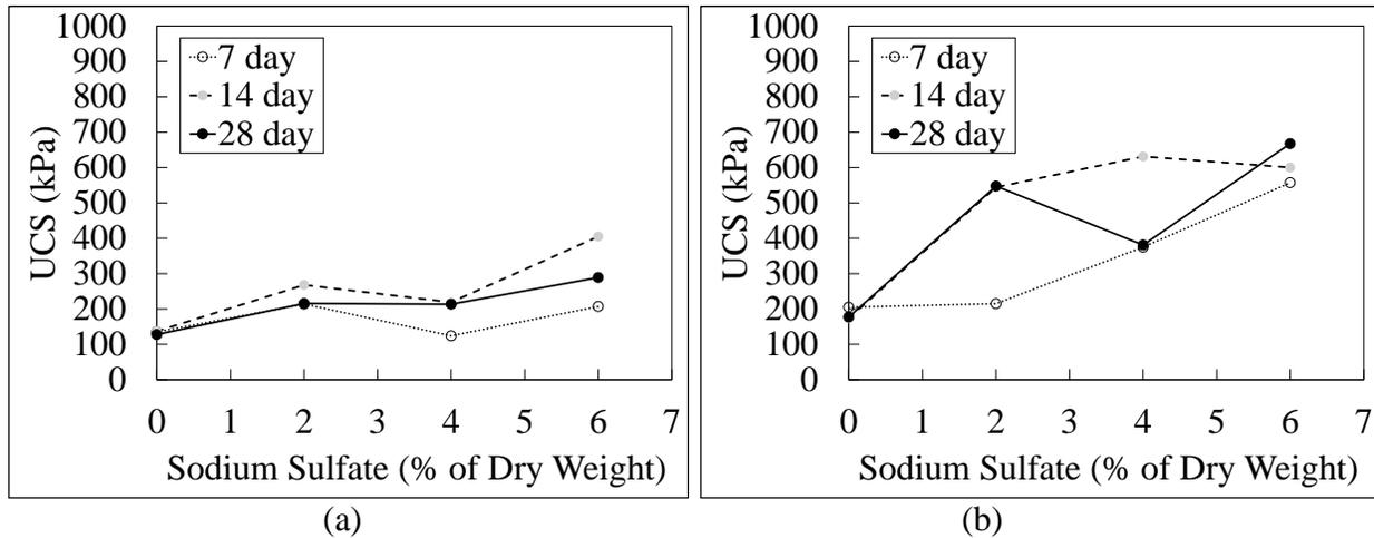
**Figure 2a. UCS of solidified fly ash (4.5% Portland cement) vs. sodium sulfate content and 2b. UCS of solidified fly ash (6% Portland cement) vs. sodium sulfate content**
