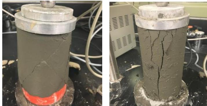
**Figure 3. Unconfined compressive strength test samples with shear (left) and tensile (right) failure**
