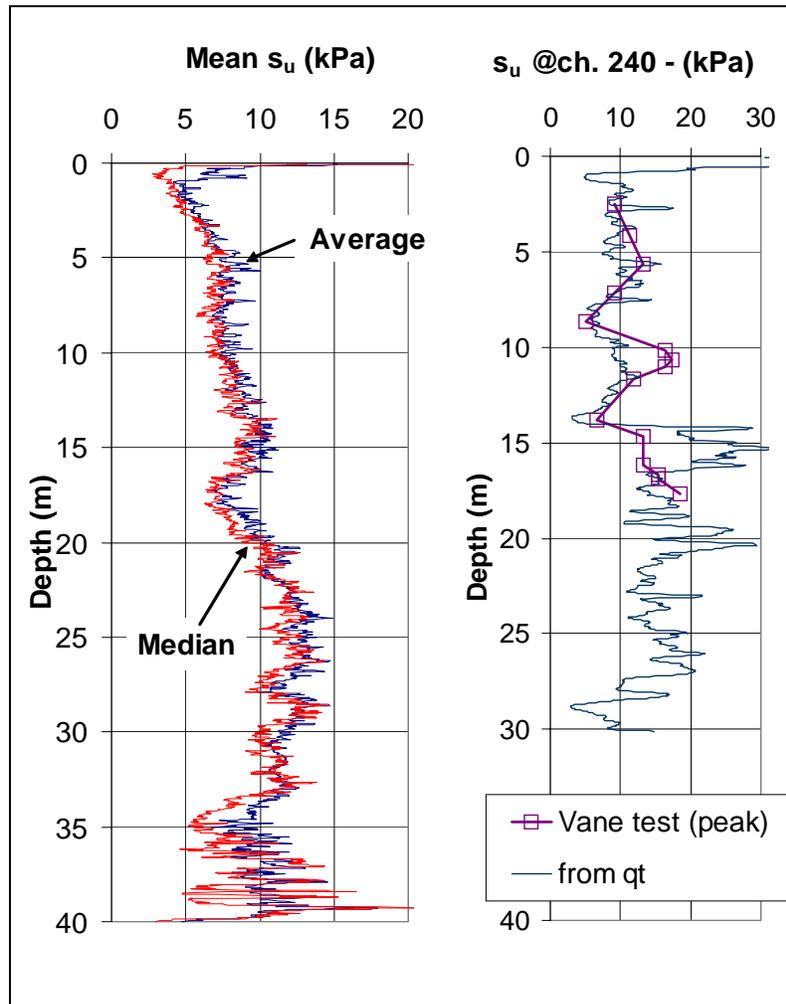
**FIG. 3 – Left, Average  $S_u$  derived from CPTu using  $s_u = 0.0486 * (q_t - u_o)$  and Right, Comparison of Field Vane data and  $S_u$ (CPTu)**
