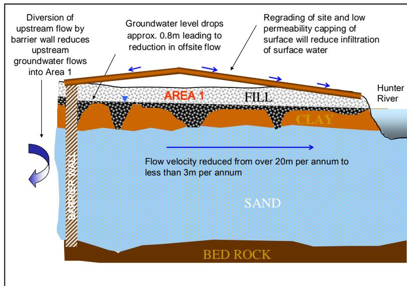
**FIG. 1. Design Concept of Containment System**
