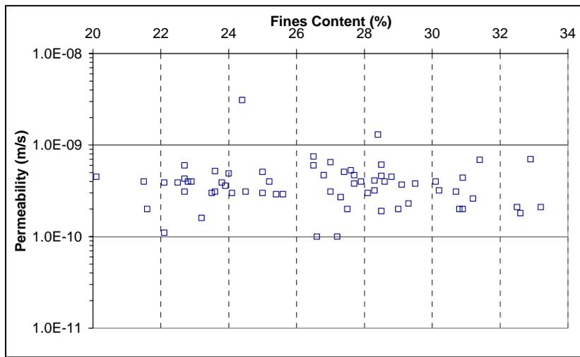
**FIG. 6. Field Samples Tested for Permeability**
