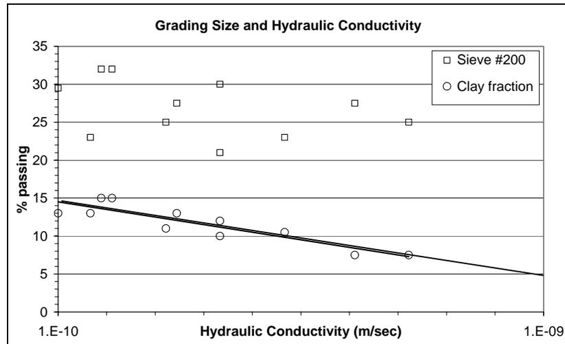
**FIG. 7. Influence of Fines Size on Measured Permeability**
