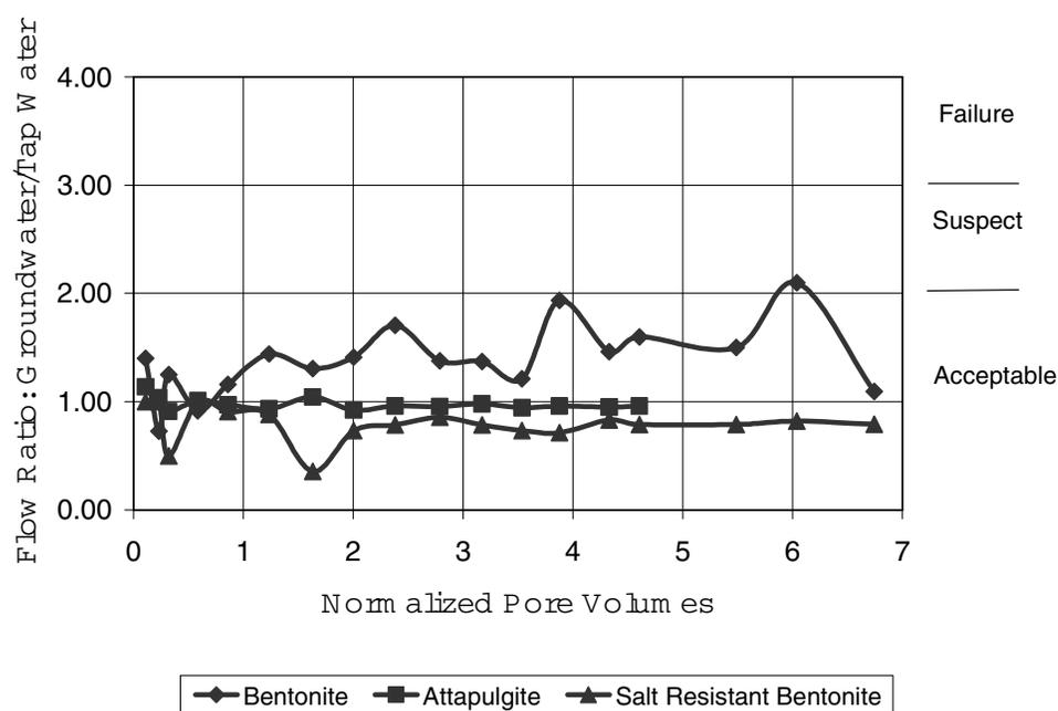
**Figure 2. Filter Press Compatibility Test Results**
