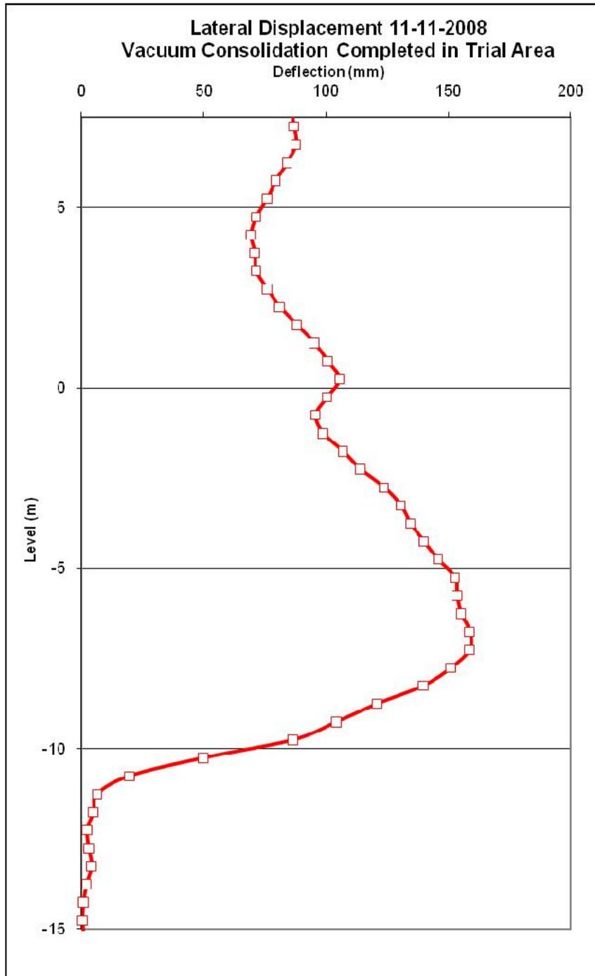
**Figure 9. Typical Inclinator Readings**
