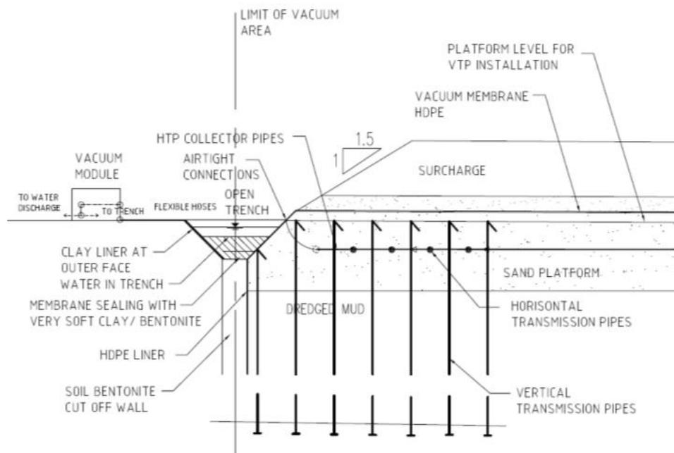
**Figure 1. Simplified cross section of Vacuum layout**
