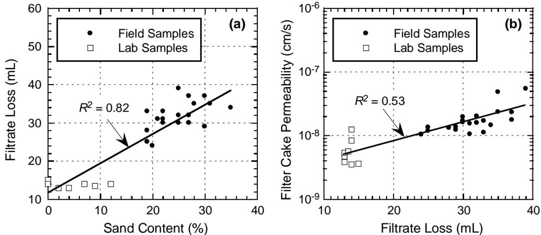
**FIG. 3. Relationship between (a) filtrate loss and sand content and (b) filter cake permeability and filtrate loss for field (in-trench) and laboratory mixed bentonite slurries.**
