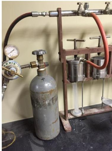
**FIG. 1. Photograph of standard filter press apparatus with carbon dioxide pressure source assembly**
