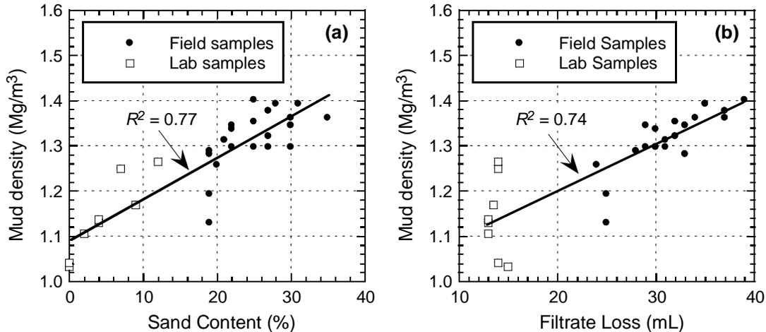
**FIG. 2. Relationship between mud density and (a) sand content and (b) filtrate loss of field (in-trench) and laboratory mixed bentonite slurries**
