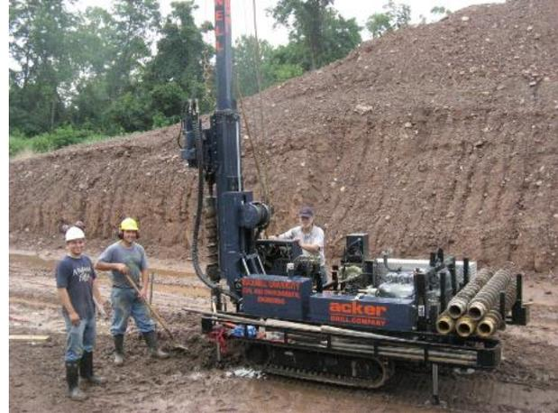
Figure 2 Drilling rig used for cutoff wall testing
