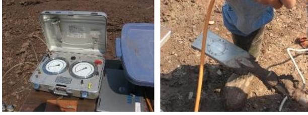
Figure 3 Dilatometer control panel (left) and blade (right)
