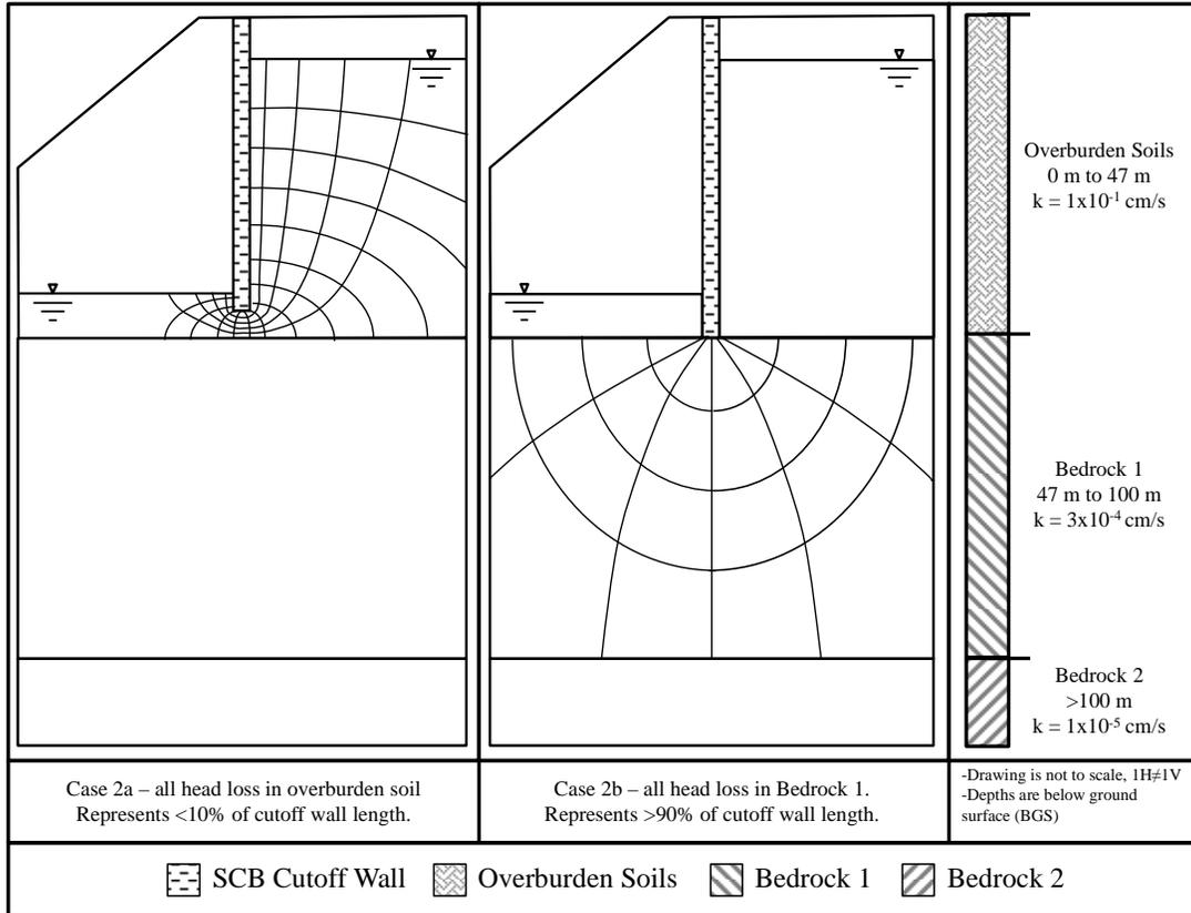
**Fig. 4. Conceptual Flow Nets for Flow through Bedrock and Overburden Soil “Windows”**
