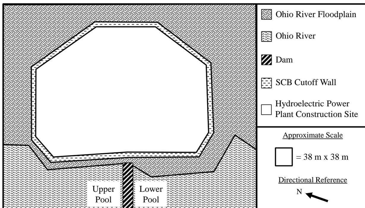
**Fig. 1. Plan View of Smithland Cutoff Wall (SCB Cutoff Wall width not to scale)**
