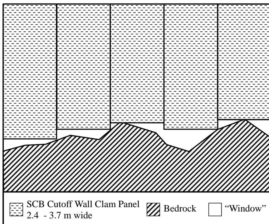
**Fig. 3. Schematic of Potential “Windows” Beneath the Cutoff Wall (not to scale)**
