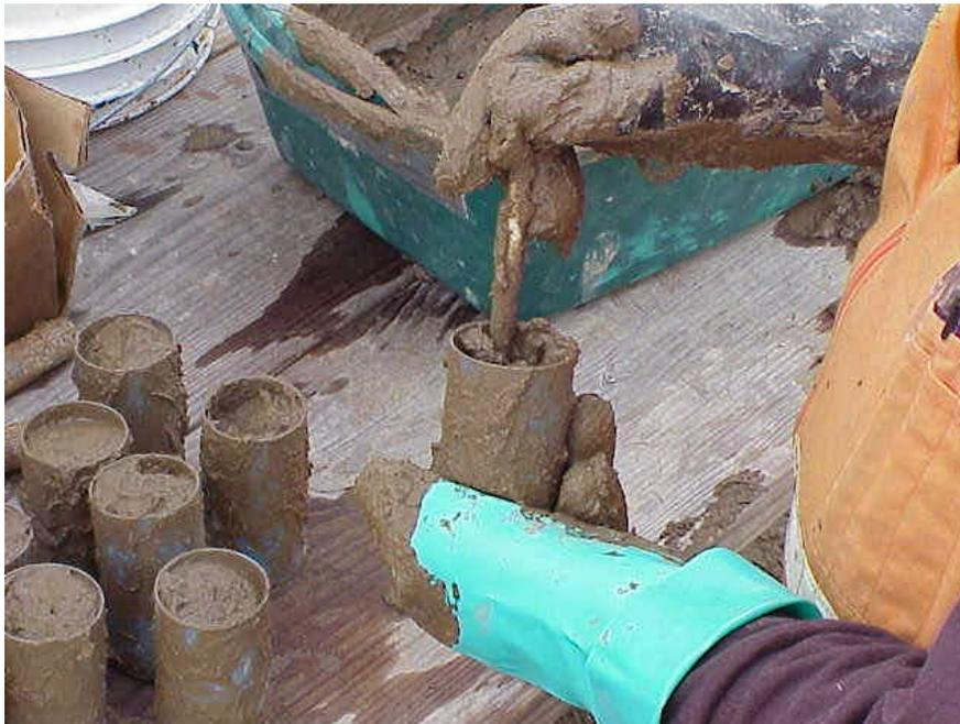
**Figure 5. Casting SCB Backfill Sample Cylinders**
