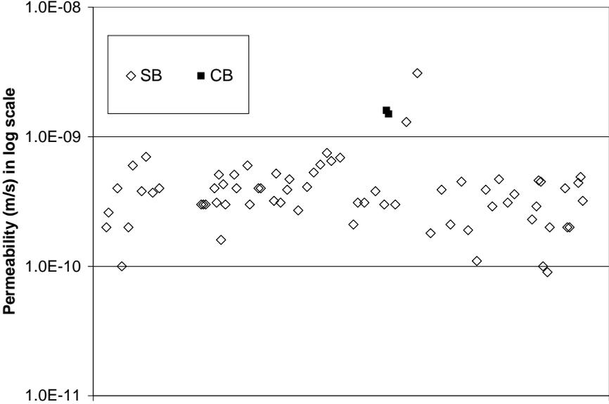
Figure 2 - Production hydraulic conductivity tests results - Mayfield
