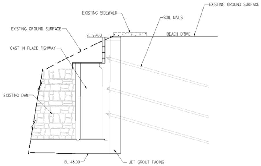
**Figure 5 - Cross Section B through Soil Nailed Wall at Dam and Beach Drive (KCI 2003)**
