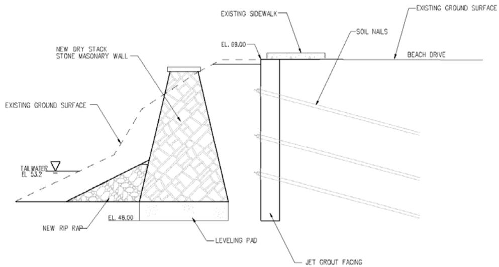
**Figure 6 - Cross Section C through Soil Nailed Wall Below Downstream Entrance to Fishway (KCI 2003)**
