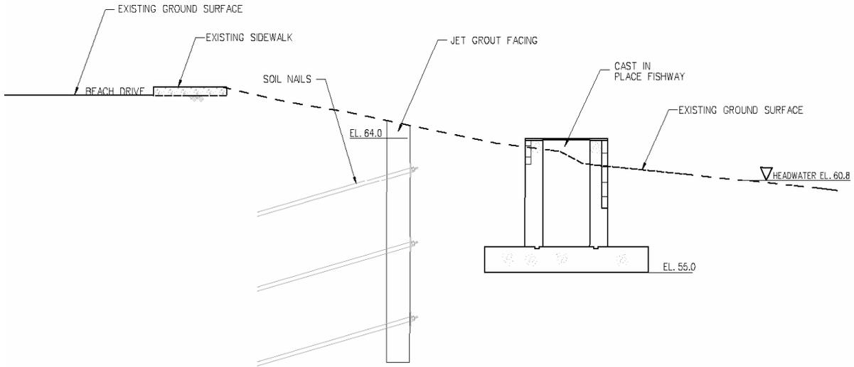
**Figure 4 - Cross Section A through Soil Nailed Wall and Upstream Exit of Fishway (KCI 2003)**
