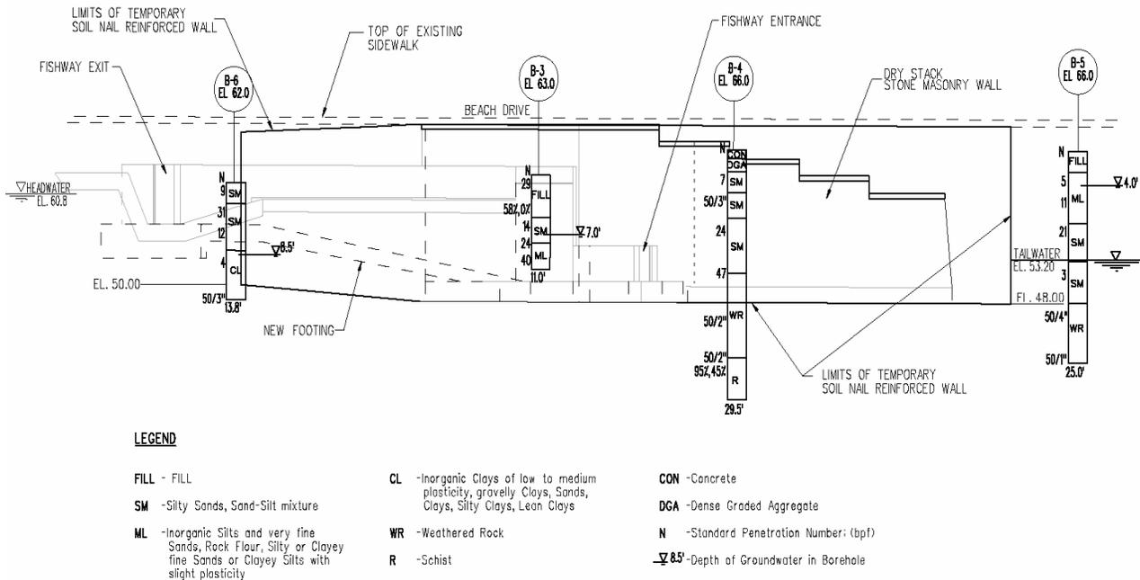
**Figure 3 – Profile of Soil Nailed Wall (KCI 2003)**
