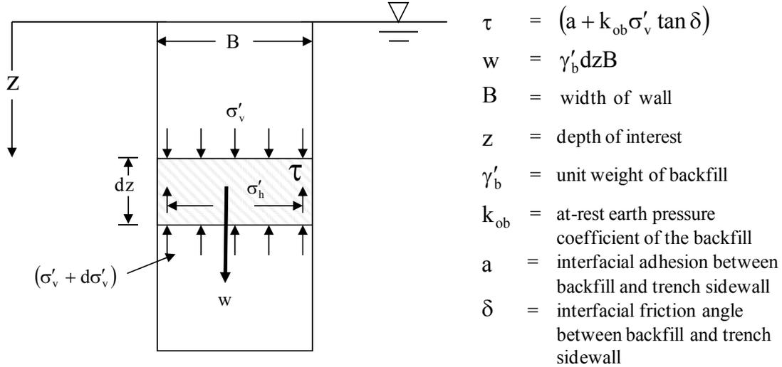
**Fig. 2. Free-body diagram for arching model (redrawn after Evans et al. 1995).**
