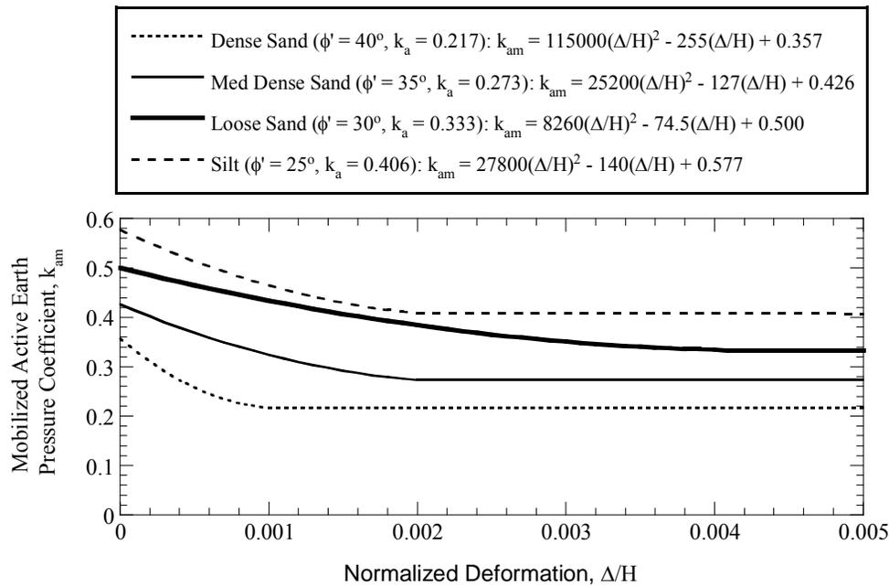
**Fig. 4. Mobilized active earth pressure coefficients ( $k_{am}$ ) plotted as a function of normalized deformation ( $\Delta/H$ ) for the four soil types in Table 1.**
