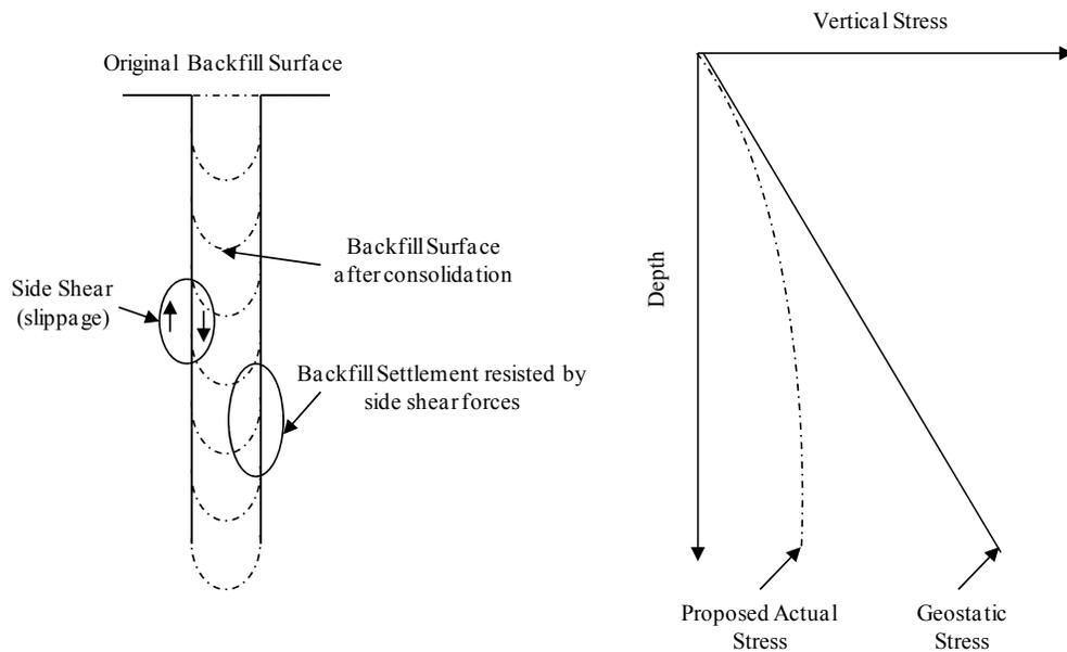
**Fig. 1. Schematic illustrating the effect of trench side friction on the stress distribution with depth in a SB cutoff wall (redrawn after Evans et al. 1985).**
