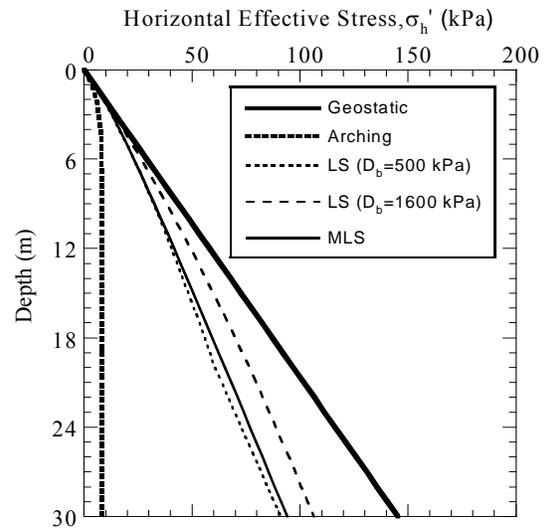
**Fig. 6. Horizontal effective stress distributions in SB cutoff wall ( $B = 1$  m) predicted by arching, lateral squeezing, and geostatic models.**
