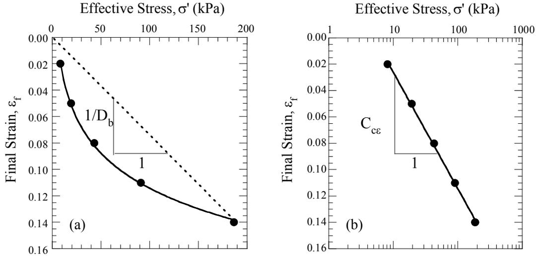
**Fig. 5. One-dimensional consolidation test results for SB backfill collected from a cutoff wall site in eastern Pennsylvania.**
