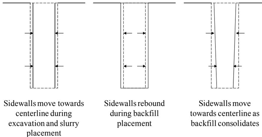
**Fig. 3. Stages of sidewall movement during construction and consolidation in an SB cutoff wall (redrawn after Filz 1996).**
