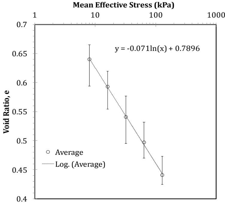
FIG. 4. Void Ratio vs. Mean Effective Stress (redrawn after Ruffing and Evans 2010)
