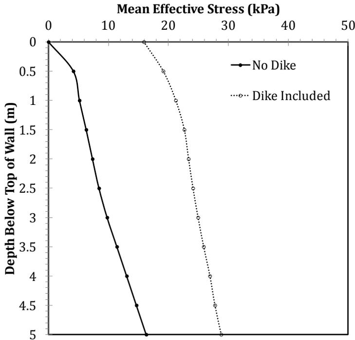
FIG. 5. Predicted *in situ* stress distribution within the backfill from MLSM
