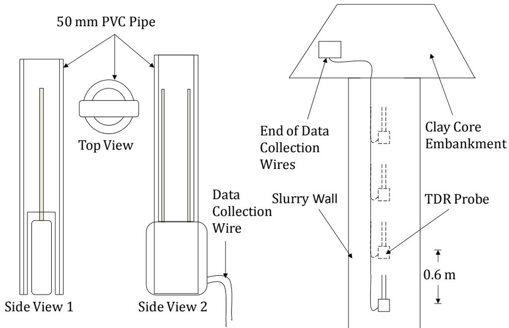
**FIG. 1. TDR sensor installation and orientation schematics**
