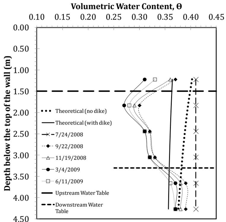
FIG. 7. Measured vs. Predicted  $\theta$  Profiles
