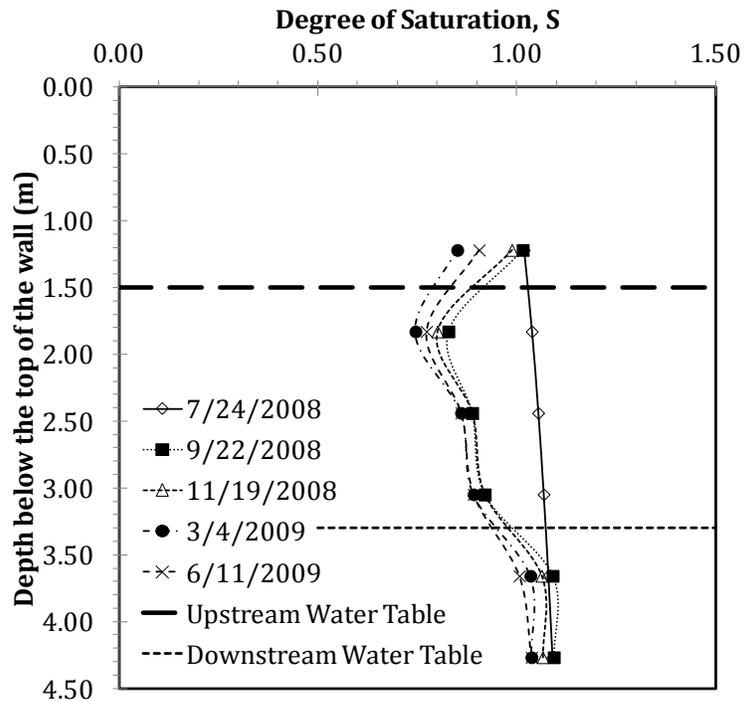
FIG. 6. Profiles of the calculated degree of saturation within the backfill
