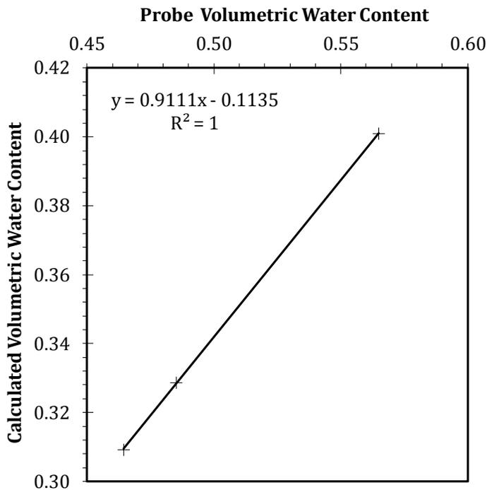
**FIG. 2. Calibration curve for TDR sensors**
