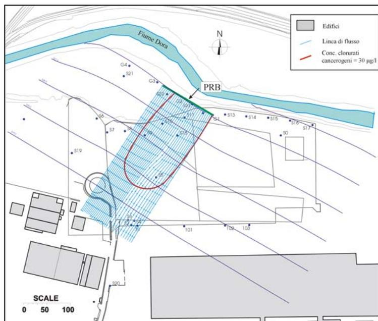
Fig. 2: Final position, orientation and capture area of the permeable reactive barrier.
