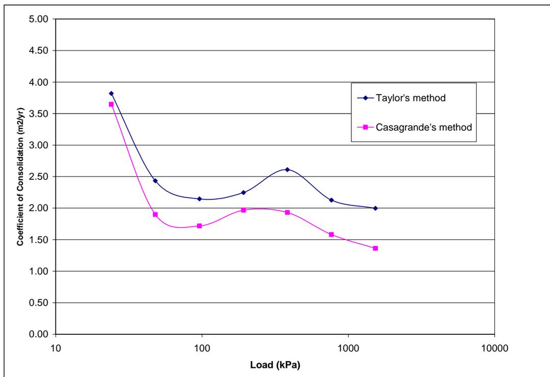
Figure 2 Coefficient of consolidation,  $c_v$ , values for SB backfill as a function of Consolidation Pressure
