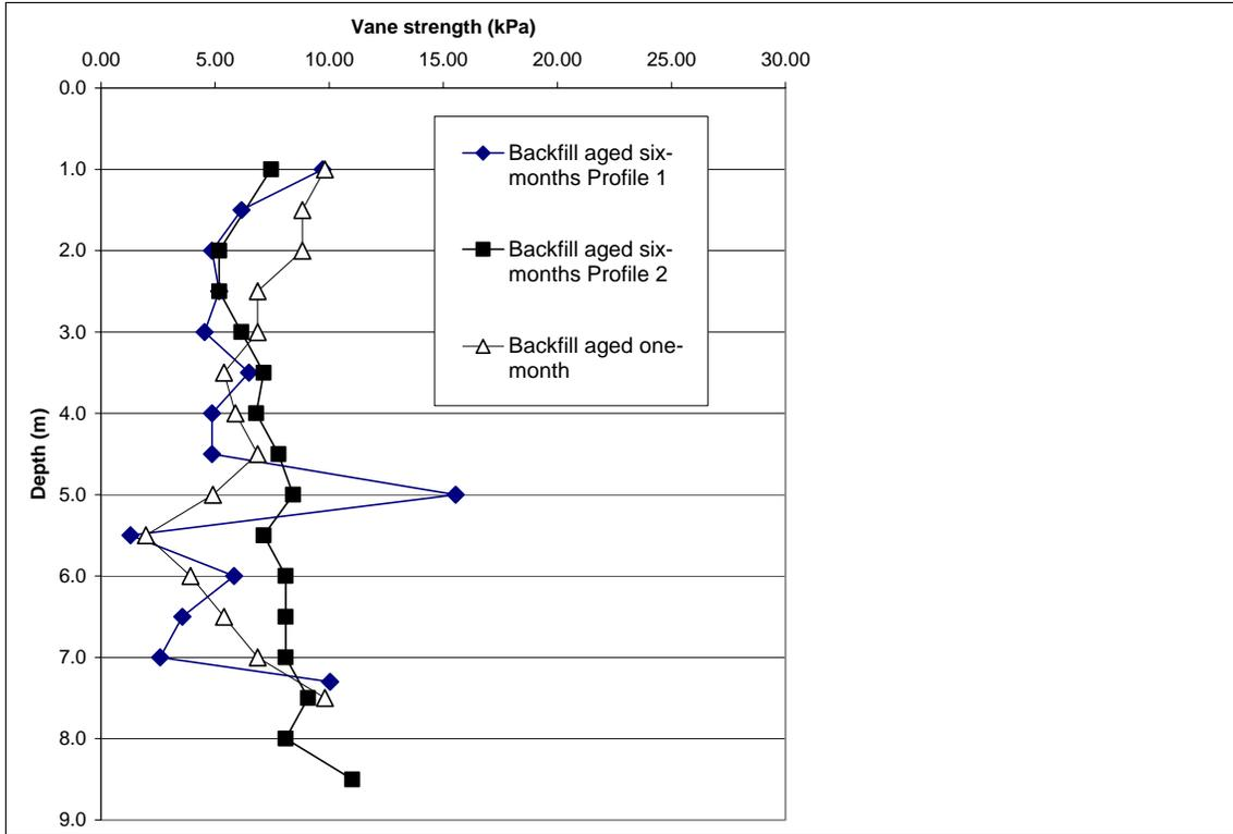
Figure 5 Vane Shear Strength of SB Backfill vs Depth
