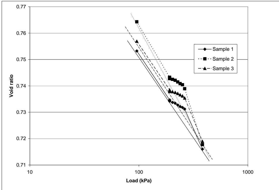
Figure 4 Quasi-preconsolidation effects in SB backfill
