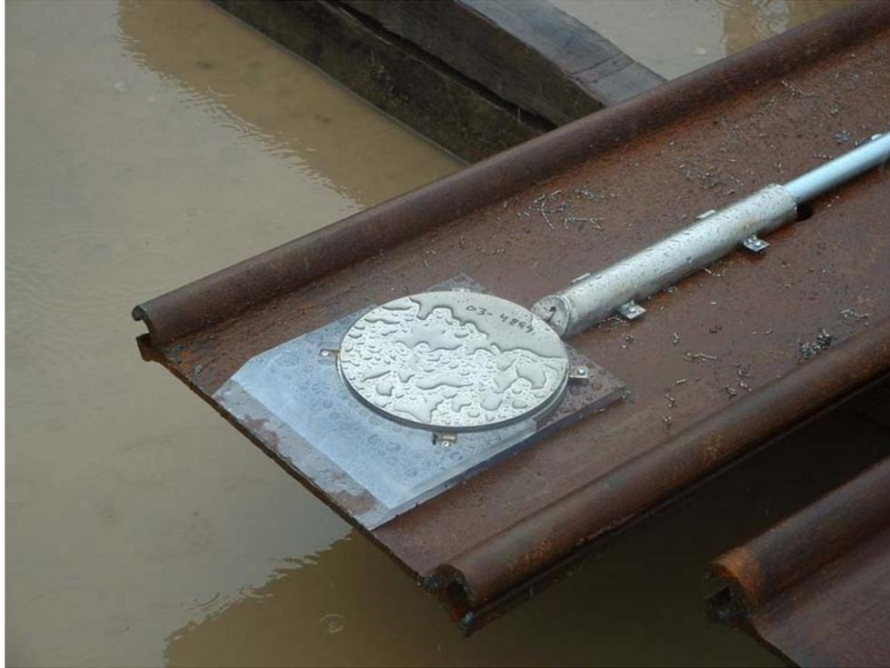
Figure 6 Earth pressure cell mounted on steel sheetpile before placement
