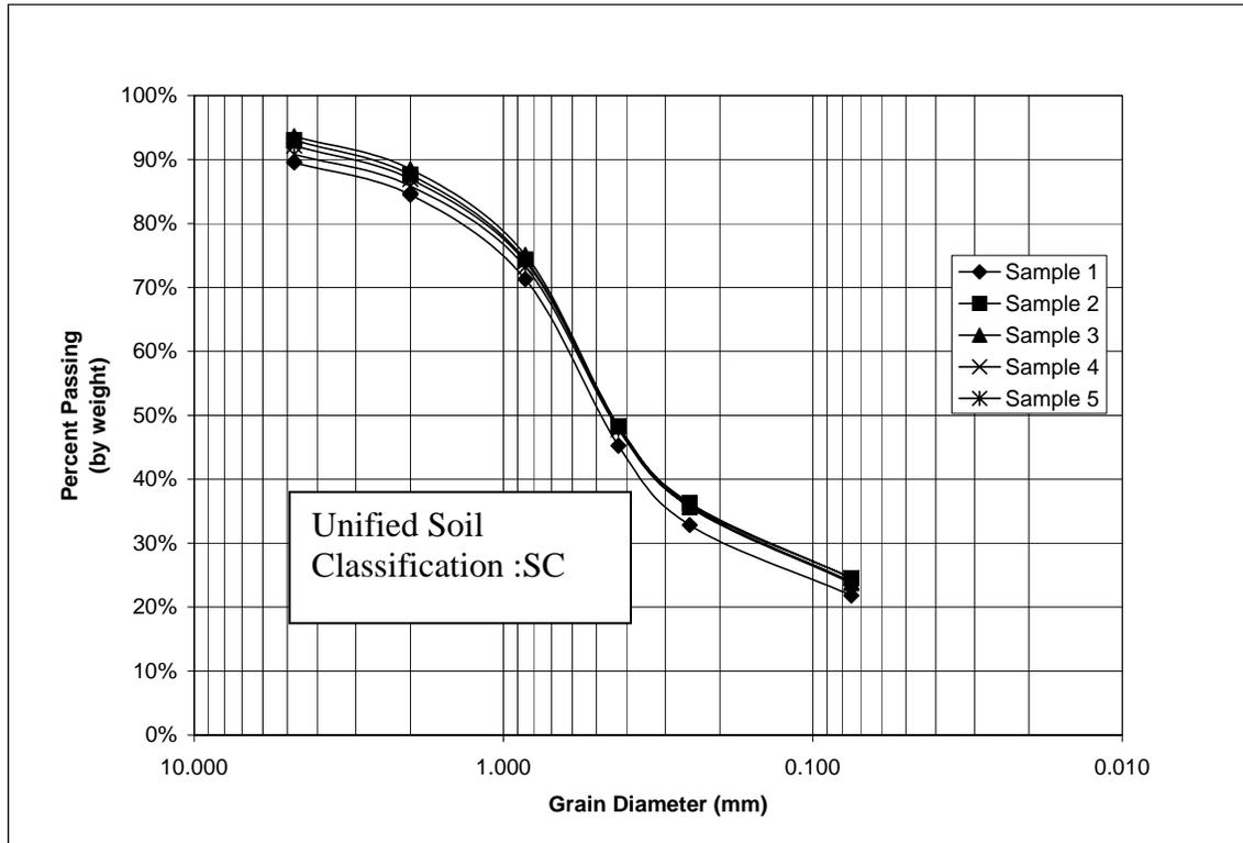
Figure 1 Grain size distribution of Delaware City backfill (ASTM D422)
