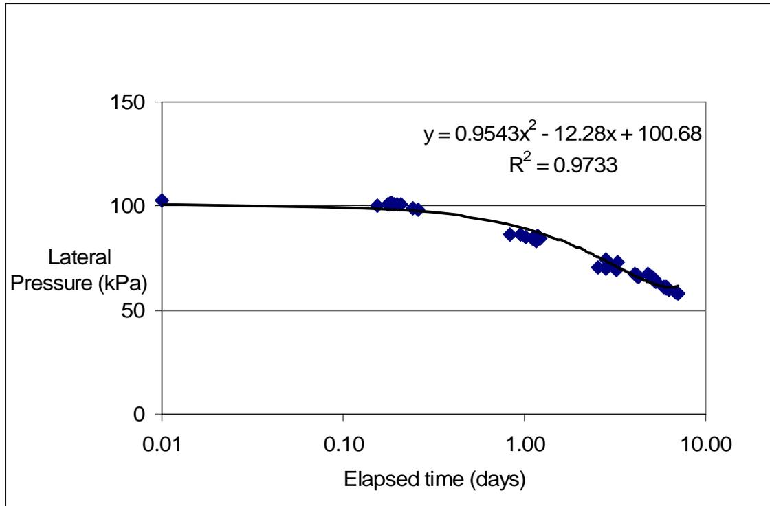
Figure 7 Time-dependent earth pressure readings in SB backfill
