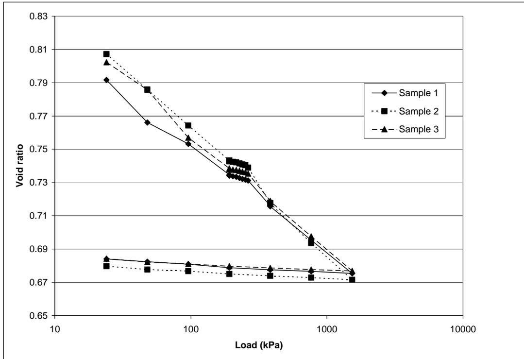
Figure 3 Consolidation test results for SB backFill
