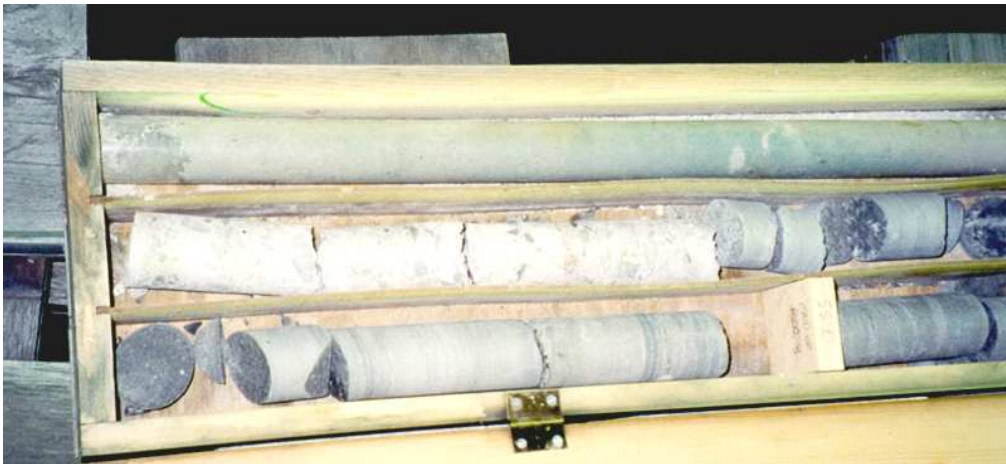
Figure 9. Confirmatory drilling core showing, from the top, grout from the tunnel, the concrete tunnel floor and bedrock.
